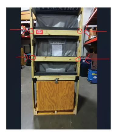
Remove the four bolts from the horizontal supports first. Then unlatch the ramp at the bottom and lastly swing the hinged bottom rail out of the way.
